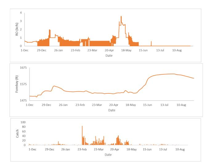
South Fork McKenzie above Cougar Dam Discharge and Cougar Dam Head of Reservoir Capture Data Since Start of Monitoring
